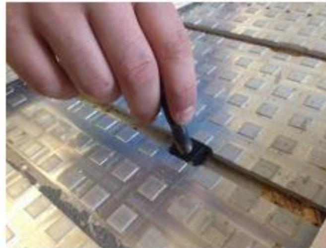
Insert clamping bolts into slots
