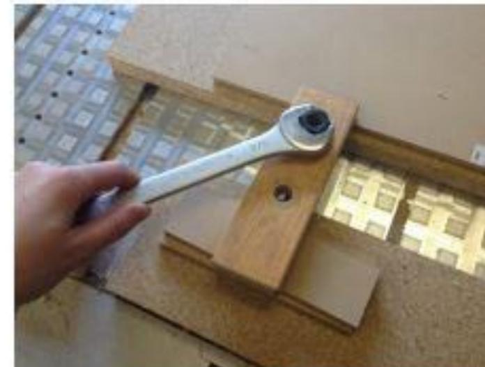
Tighten the bolts to secure the stock
